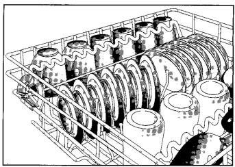
Items can be centered behind a single tine or loaded at an angle to maximize space. For best results, leave a small space between pieces so they do not touch during the cycle.
